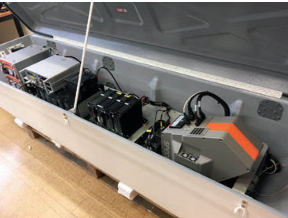
Above: Custom built mount for the airborne MSIR system. Left: Components of the airborne MSIR system.
