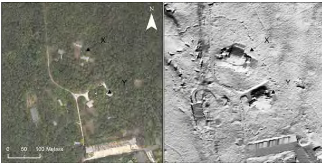
Figure 3: The visible image on the left reveals little about the features lying beneath trees at locations X and Y, whilst lidar (right) shows the presence of two domed features.
