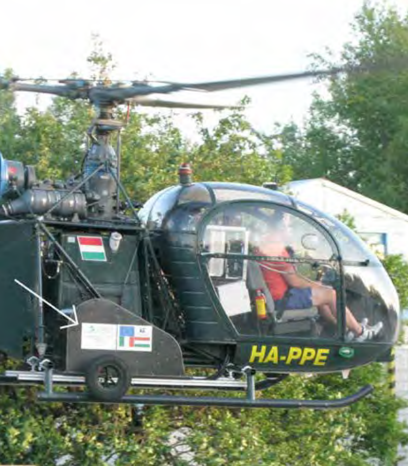
Image 1: Tests so far have involved mounting MSIR sensors in an external pod (see white arrow pointing to black box above wheel) on a relatively small helicopter but future tests will involve larger aircraft types.
