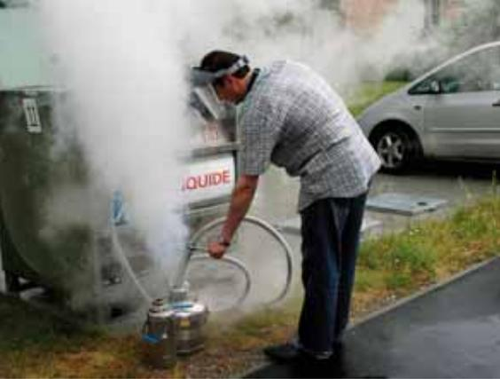
Above: Filling a dewar with liquid argon for cooling the ARIX-3F system.
