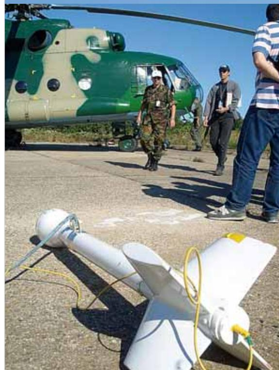
2006 directed exercise, Croatia: magnetometer for towing underneath helicopter.
