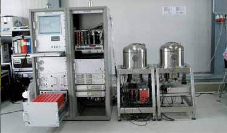
Above right: SAUNA laboratory unit for analysis of xenon samples taken in the field. The system was developed for OSI and tested in Seibersdorf, Austria, in July–September 2006.
