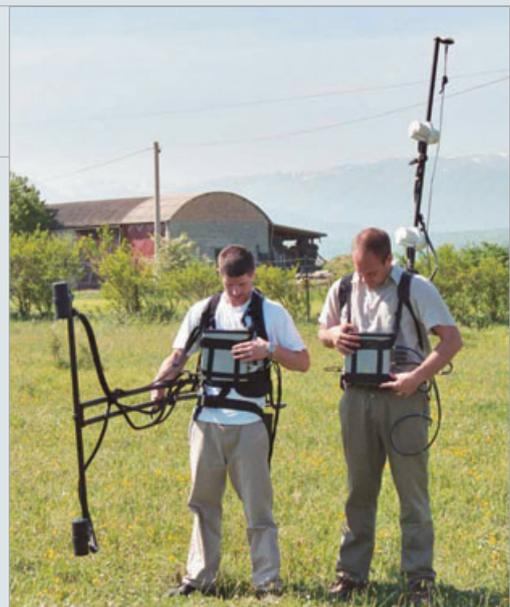
*OSI equipment demonstration, Italy: magnetometers.*
