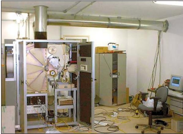
*Automatic particulate air sampler (RASA) installed at radionuclide station RN11, Rio de Janeiro, Brazil.*
