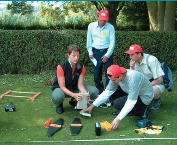
*OSI equipment demonstration, United Kingdom: assembly of a ground penetrating radar system prior to use in the field.*
