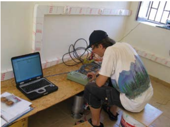
INFRA SOUND OFFICER PERFORMING MICROBAROMETER COMPARISON TEST (PART OF THE CERTIFICATION MEASUREMENTS)
