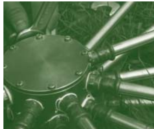
DETAIL OF AN INFRASOUND ARRAY
