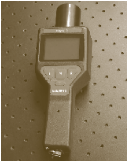
HAND-HELD RADIONUCLIDE SURVEY AND ANALYSIS TOOL
