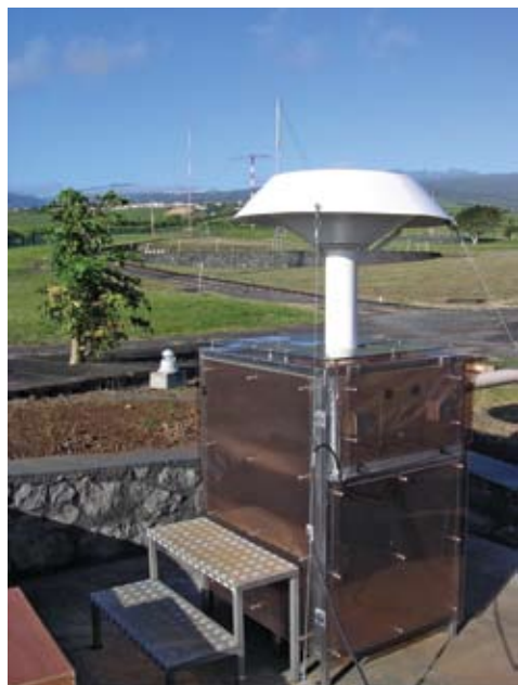
MANUAL STATION AIR SAMPLER AT RN29, RÉUNION, FRANCE
