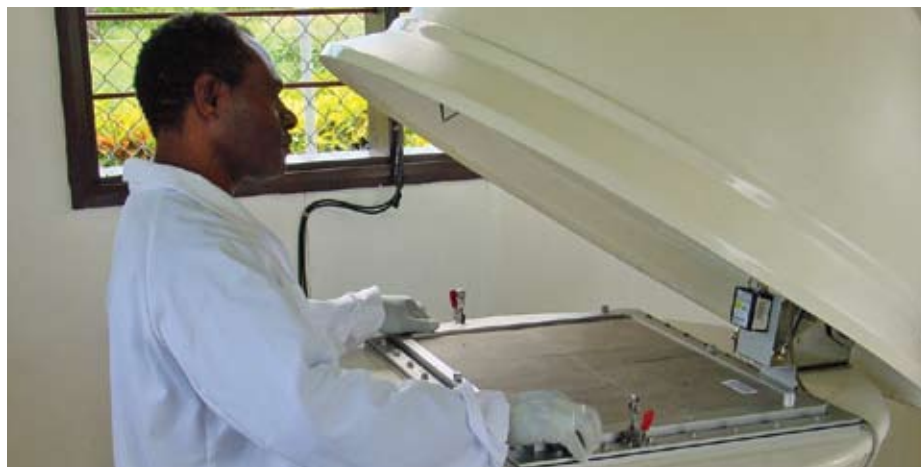
DAILY CHANGE OF FILTER IN THE AIR SAMPLER AT RN51, NEW HANOVER, PAPUA NEW GUINEA
