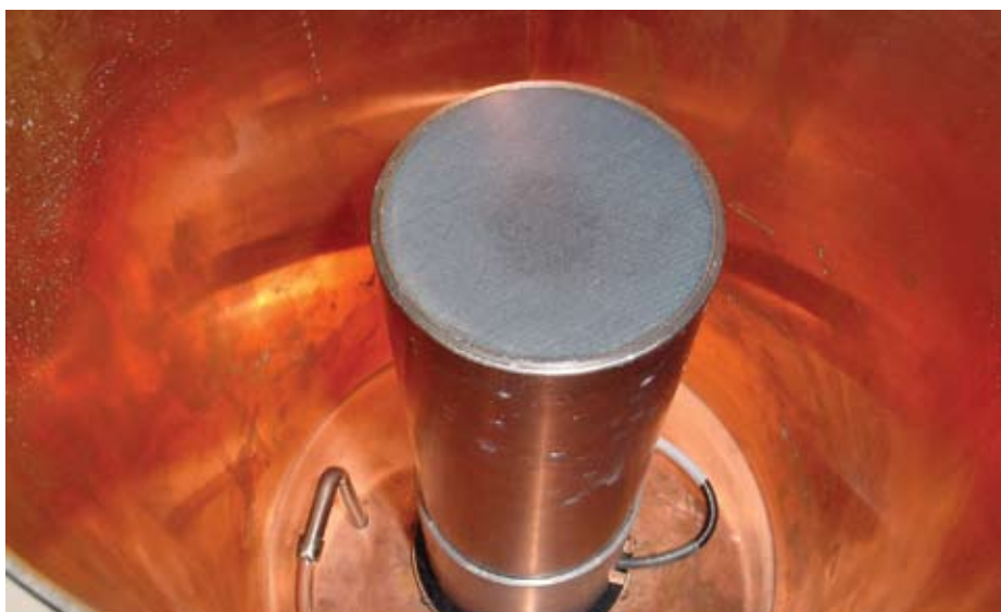
HIGH-PURITY GERMANIUM DETECTOR IN ITS LEAD SHIELD WITH AN INNER COPPER LINING
