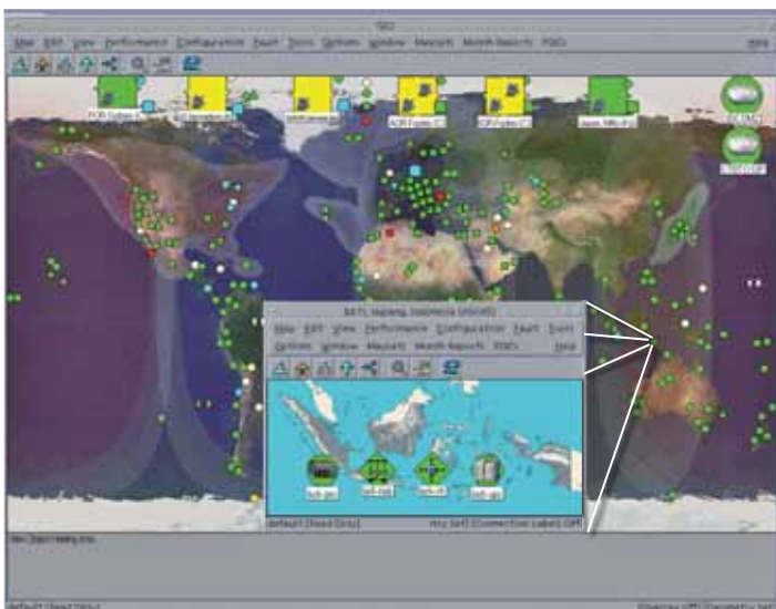
SCREENSHOT OF GCI NETWORK MANAGEMENT SYSTEM DISPLAYING REAL TIME STATUS OF GCI LINKS
