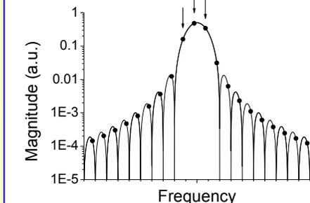
Theoretical spectrum of one sinusoid (dots mark discrete Fourier transform).
