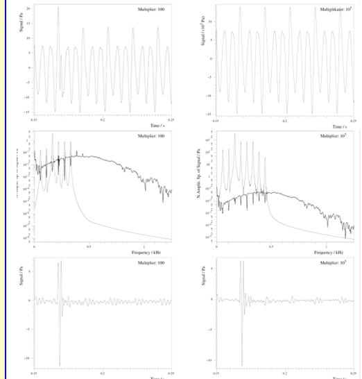
Impulse superposed with line series (8 lines, 55-440 Hz). Multiplier 100 (left column),  $10^7$  (right column). Top: signal; centre: spectrum, found and fitted lines, subtracted spectrum; bottom: back-transformed time signal.
