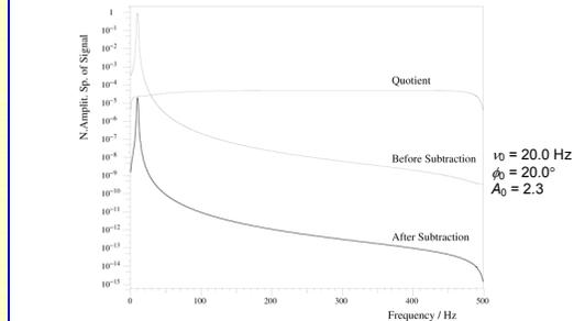
Original spectrum of one sinusoid ("Before Subtraction"), remaining difference after subtracting theoretical spectrum of line with parameters from fit ("After Subtraction"), and quotient of both. The difference is due to slight deviations of the fitted parameters. Lines are fitted and subtracted one after the other, ranked by amplitude.
