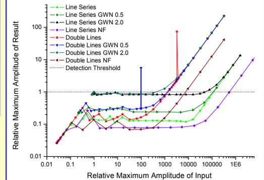
Peak-to-peak value of corrected signal before the impulse divided by p-p-value of impulse versus the same ratio before correction.
