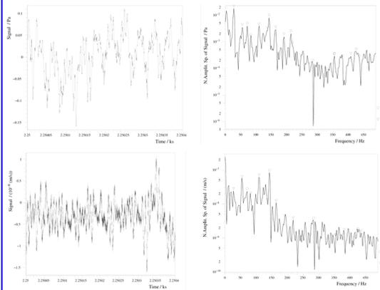
Signal (left) and spectrum (right) of a landed helicopter at about 1 km distance. Top: acoustic, bottom: seismic. In the spectra two harmonic series can be found stemming from the main (triangles) and the tail (circles) rotor, respectively.
