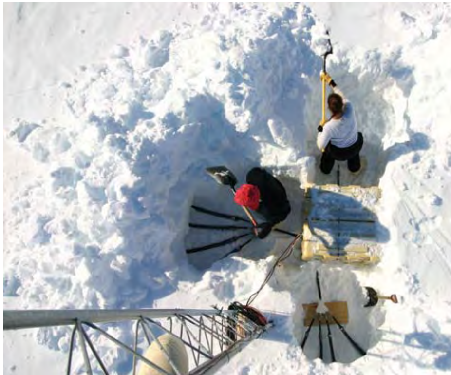
DIGGING OUT THE WIND NOISE REDUCING PIPE ARRAY AND EQUIPMENT VAULTS AT IS55. PHOTO COURTESY OF DUNCAN MARRIOTT, GEOPHYSICAL INSTITUTE, UNIVERSITY OF ALASKA, FAIRBANKS.
