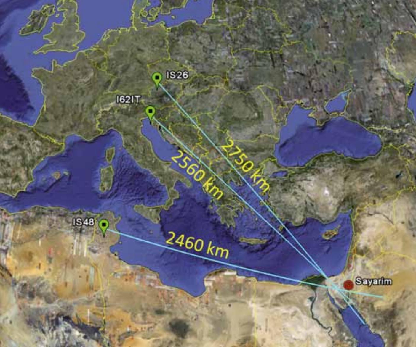
Location of Sayarim Military Range in Israel. IMS detecting stations IS26, (5 elements, Freyung, Germany), IS48 (8 elements, Kesra, Tunisia) and the CTBTO's portable array I62IT (4 elements, Strassoldo, Italy). Blue lines represent the back-azimuth extracted from the detected signals for each infrasound array.
