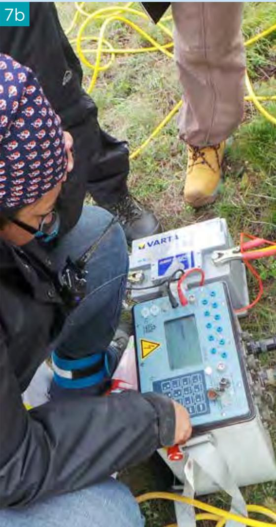
**7a** Various geophysical methods such as geoelectrics were also utilized by the inspection team. These OSI techniques can detect underground anomalies caused by an underground nuclear test or its preparations.
