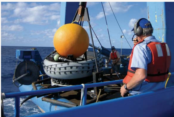
HYDROPHONES – UNDERWATER MICROPHONES – ALONG WITH BUOYS TO KEEP THEM AT A CERTAIN DEPTH, ARE BEING DEPLOYED INTO THE SEA.
