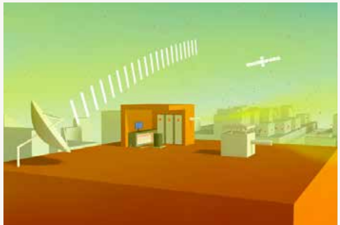
RADIONUCLIDE STATIONS CAPTURE AIRBORNE PARTICLES FOR ANALYSIS TO IDENTIFY THE RADIOACTIVE ELEMENTS, OR RADIONUCLIDES, THEY CONTAIN.
