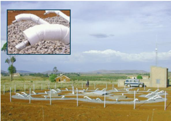
VIEW OF WIND NOISE REDUCING PIPE ARRAY AT AN ARRAY ELEMENT OF INFRASOUND STATION IS33, ANTANANARIVO, MADAGASCAR. INSET: INLET PORTS OF PIPE ARRAY.
