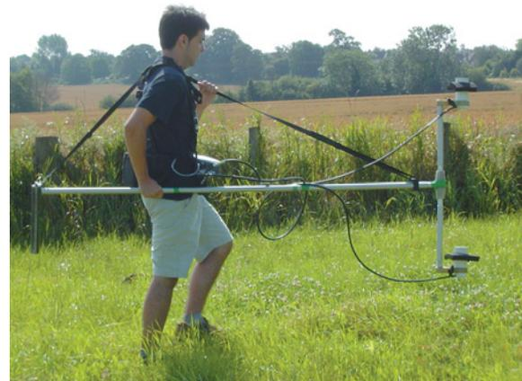
*OSI equipment demonstration, United Kingdom: magnetic field mapping survey with a caesium vapour magnetometer.*
