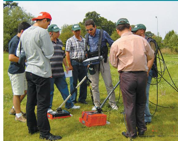
*OSI equipment demonstration, United Kingdom: demonstration and testing of two alternative ground penetrating radar systems.*
