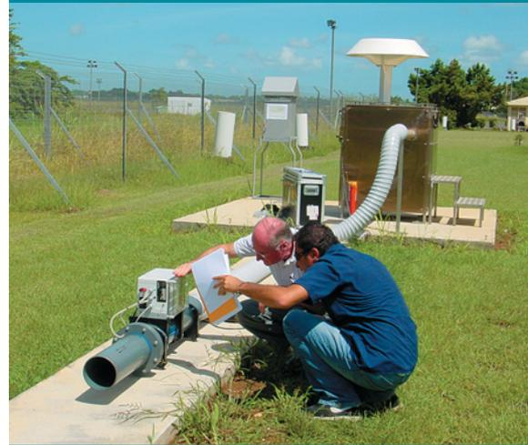
*Airflow measurement check of manual particulate air sampler at radionuclide station RN28 Pointe-à-Pitre, Guadeloupe, France.*
