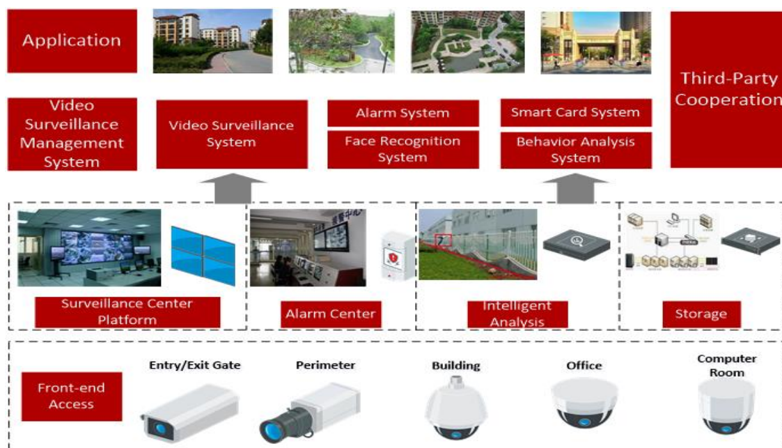
Figure 4.1 Video Integrated Management Platform Architecture Design
