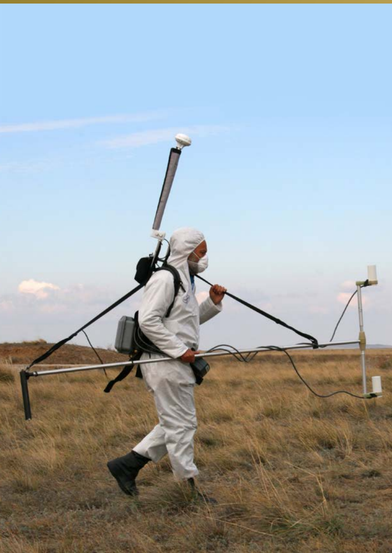
An OSI specialist carries a magnetometer, an instrument that measures deviations in the Earth's magnetic field and helps to identify cavities that may have been caused by an underground nuclear explosion
