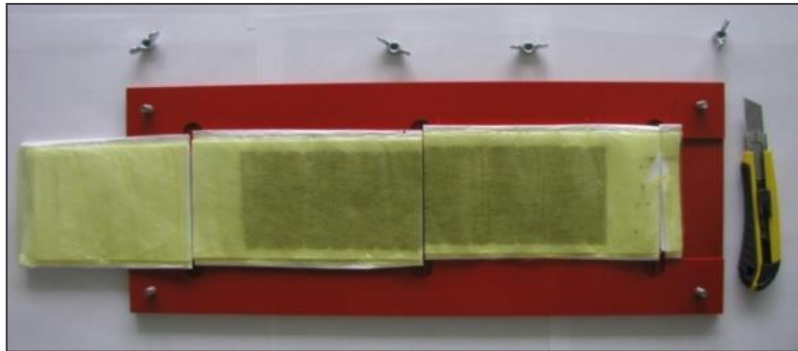
Figure 6. Splitting of the full RASA sample at a station. A cutting tool is used.
