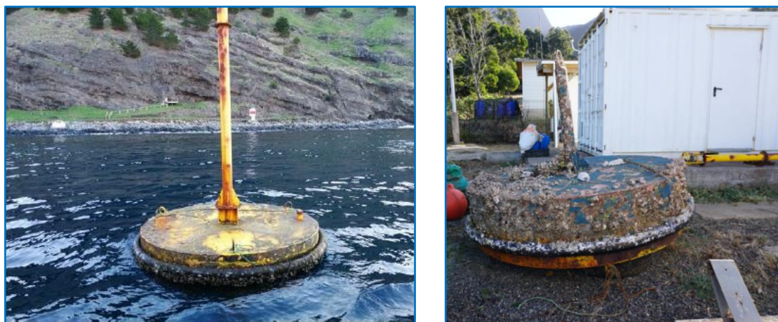
Figure 2: Buoy shortly before (left) and after (right) its recovery during the 2019 rotation. Note that the photograph on the right shows the buoy in an upside-down position and before anodes and marine growth were removed; the detached topmast is visible in the background.
