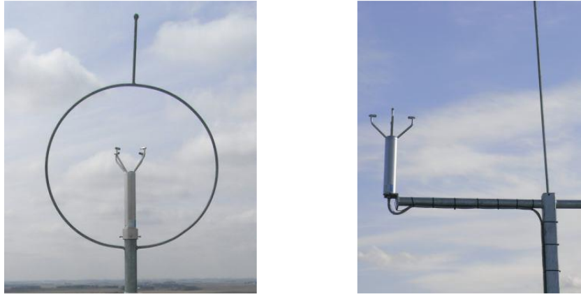
Figure 55: Examples of lightning rods providing sufficient area of protection for a met sensor
