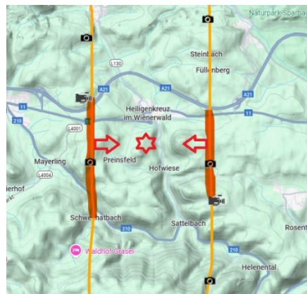
Figure 3 Drawing of how a sketch could look like when the same observable is filmed with left/right-looking cameras as the airframe flights back along the next flight line.
